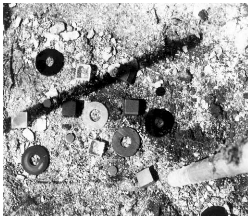
Fig. 3. SRS glass samples being buried at Ballidon, UK.
